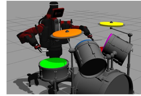
We synthesise sound to coincide with drum collisions and integrate this with recorded joint angle and camera data.
